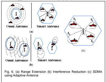
Furthermore, smart antennas provide maximum flexibility by enabling wireless network operators to change antenna patterns to adjust to the changing traffic or RF conditions in the
