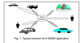
For mobile applications, the directivity of the antennas has to be adapted such that the beams pointing to the users can follow their movements. This is called adaptive SDMA or A-SDMA. An example of a typical A-SDMA scenario is depicted in Fig. 1, where seven mobile stations are served on only two carrier frequencies marked by bright and dark beams, respectively [27].
